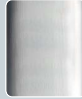
Rohr komplett geschliffen tube grinded completely
